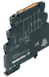
The solid-state relay **MICROOPTO ACTOR** has been specifically designed as a switching amplifier for actuators up to 24 V DC and 2 A with inductive loads such as solenoid valves and contactors. 2-wire actuators can be connected directly to the module. This is short-circuit proof and protected against application-related transients and spikes by extensive protective circuitry.
