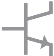
**Bipolar transistor (for DC outputs)**
