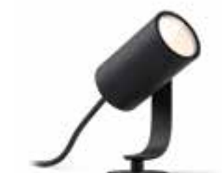
8718696167977 Lily spike anthracite extension 1 192 → 84 ↗ 70 mm 8 W, 640 lm at 4 000 K, 2 000–6 500 K PSU needed (p. 54)
